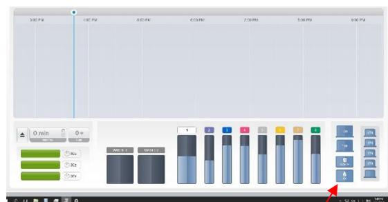
Operators can refer to the Graphical User Interface for indications of solvent availability in the coverslip activator bottle.
