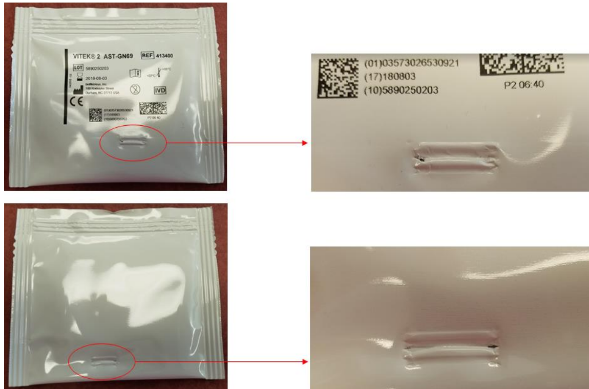
Figure A - Example of Pouch Defect
