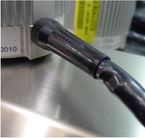
Figure 5: Cable Damage at the Motor Bend Relief
