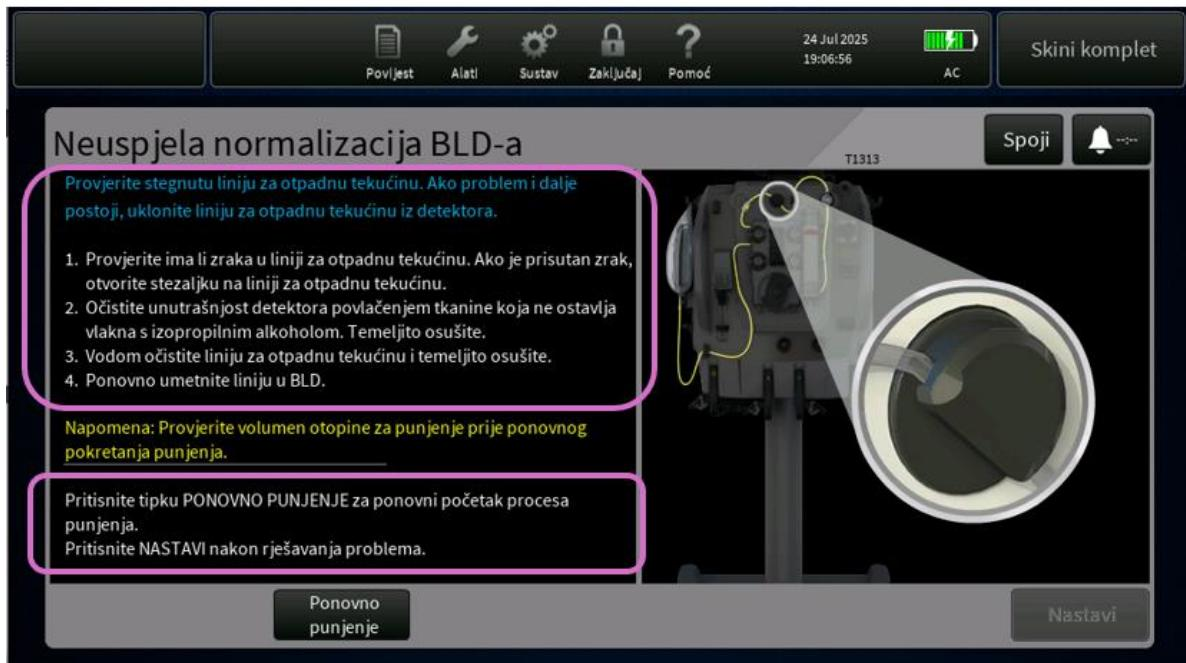
The Alarm Screen guides the user in resolving the BLD Normalization failure and provides possible next steps – *Reprime* or *Continue*.
