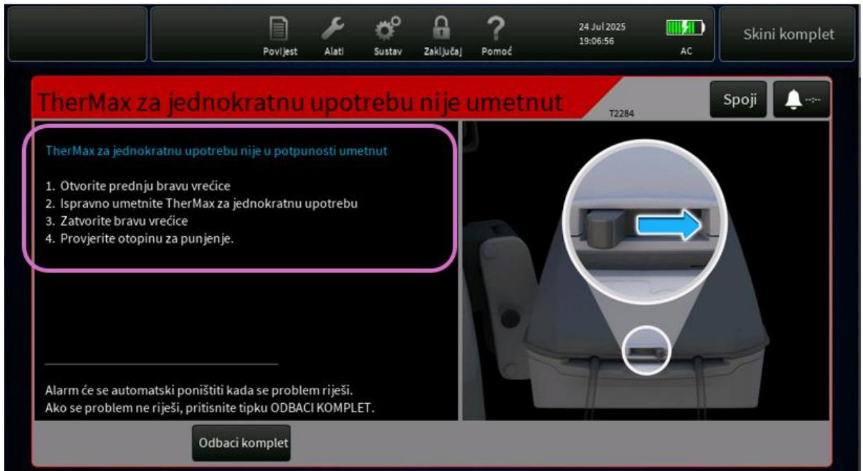
The Alarm Screen guides the user in resolving TherMax disposables detection issue and provides an option to *Discard Set* if the problem is not cleared.
