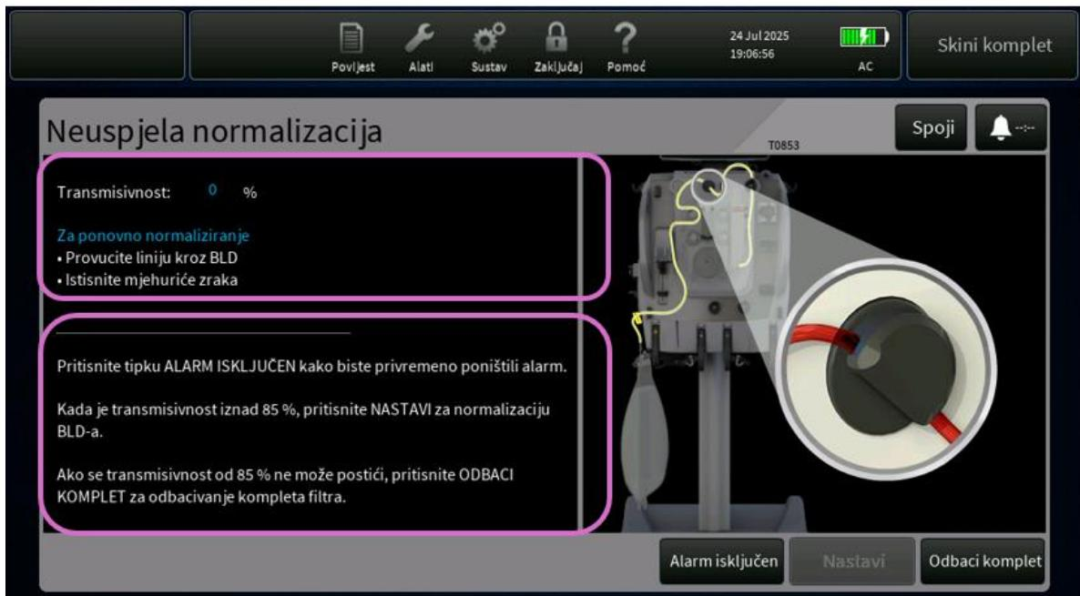
5. **Alarm T1205 : BLD Self-Test Failure** – The PrisMax system displays the following Alarm Screen when the alarm *T1205 : BLD Self-Test Failure* is active.
