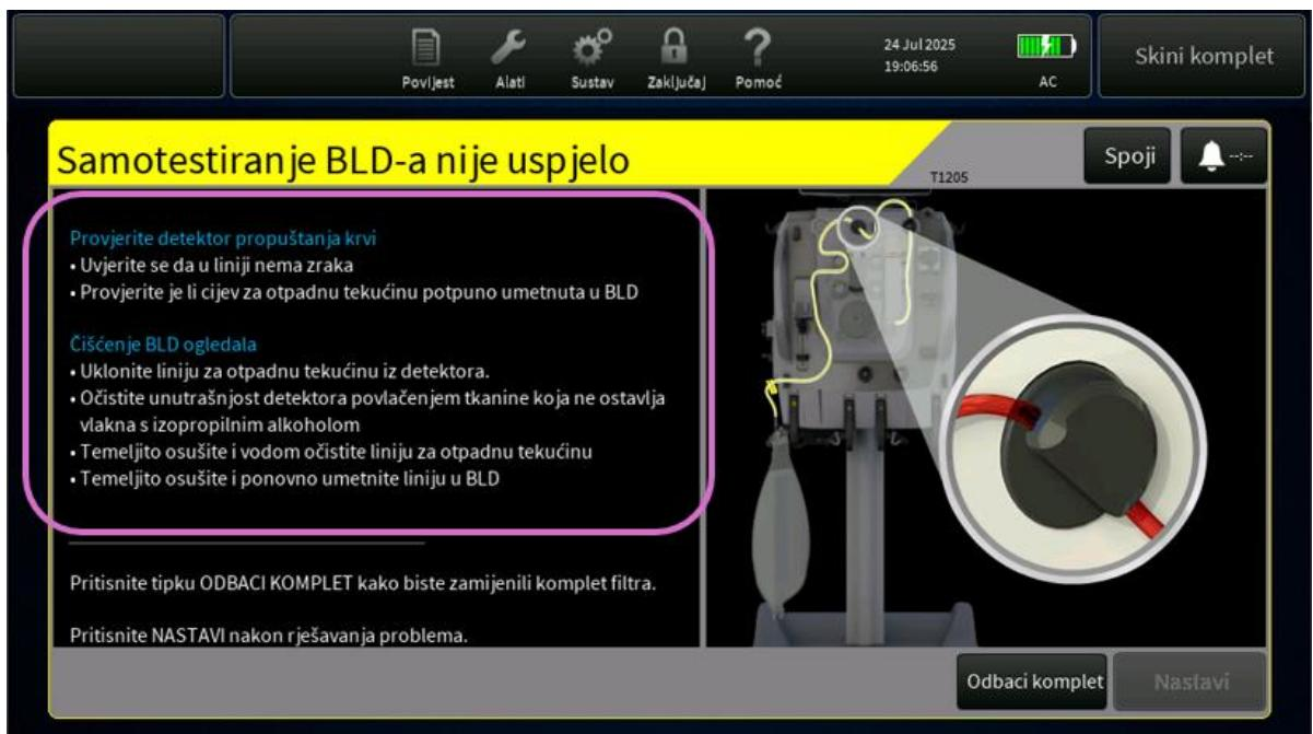
The Alarm Screen guides the user to investigate potential source of BLD Self-Test Failure and provides next steps – *Discard Set or Continue*.
