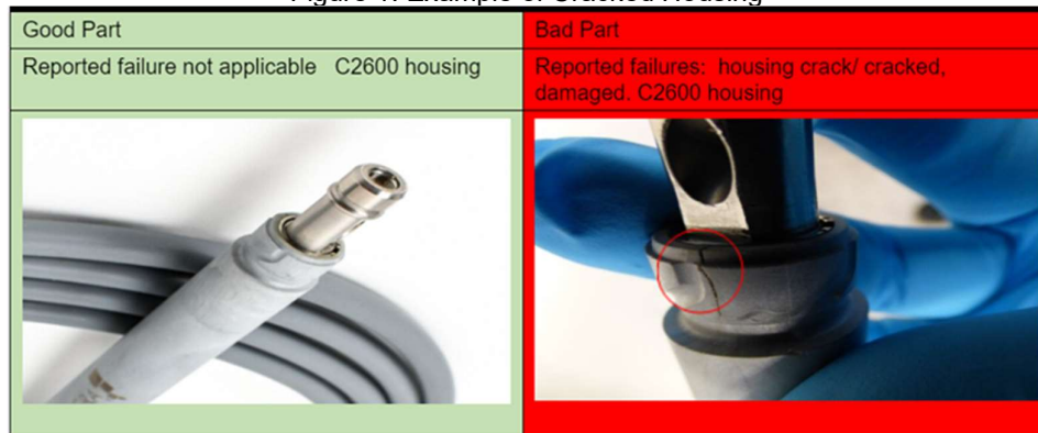
Figure 1: Example of Cracked Housing
