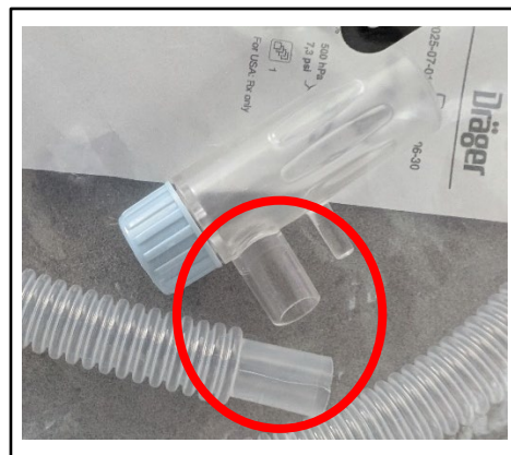
Fig. 2: Detached hose/ PEEP valve
