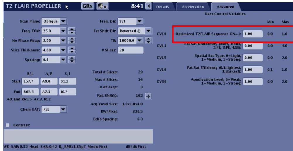
Figure 4. Optimized T2 FLAIR Sequence enabled (set to 1.00) in the Advanced Tab for T2 FLAIR Propeller
