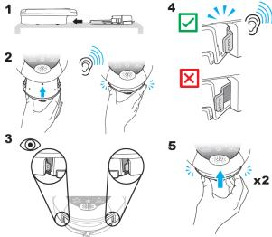
Illustration 5: Push the Pad-Pak in one last time to ensure correct engagement. Once you've verified proper insertion, return the device to its storage location for use.
