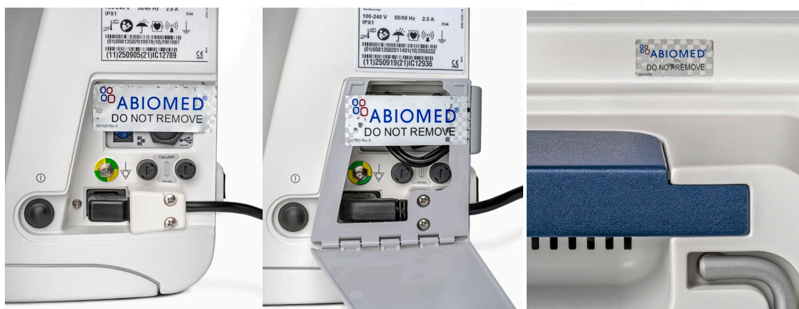
Figure 2. Automated Impella Controllers with evidence of tampering.
