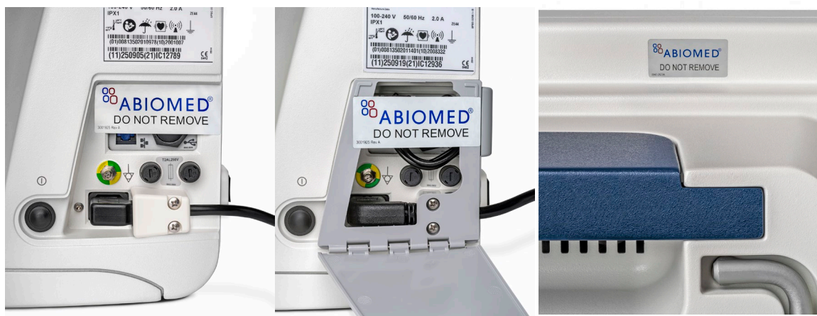
Figure 1. Automated Impella Controllers without evidence of tampering.
